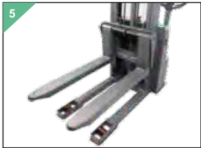
Fixed legs with adjustable forks
