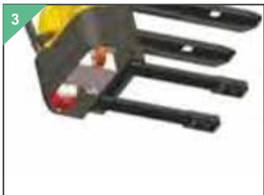
4-point design, improve the trucks' stability
